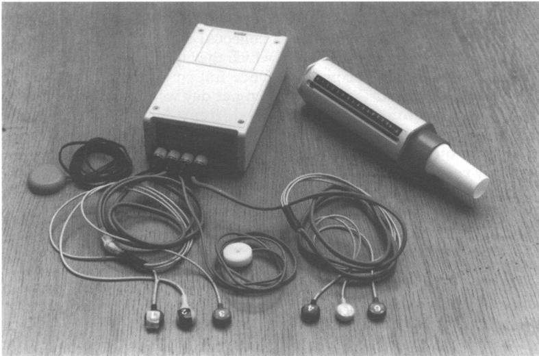
Figure 1 RBC-7 Multiparametric recording device (with peak expiratory flow meter for size comparison).
