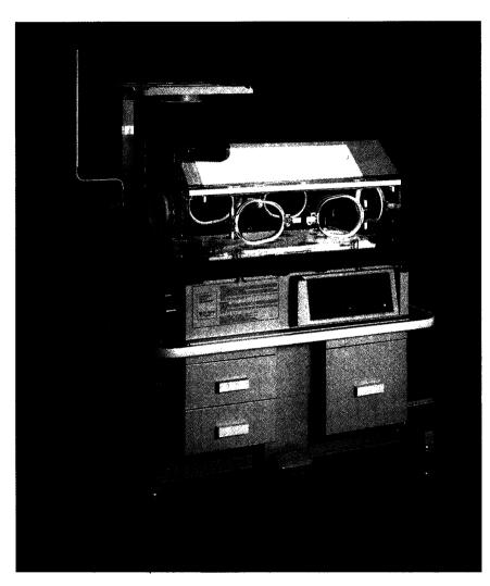
With the touch of a foot pedal, the new Variable Height Adjustment (VHA) mechanism on the C100 Quiet Touch allows continuous control of the baby's level from a towering 43 inches to a low 34.5 inches — just right for a comfortable armchair.
