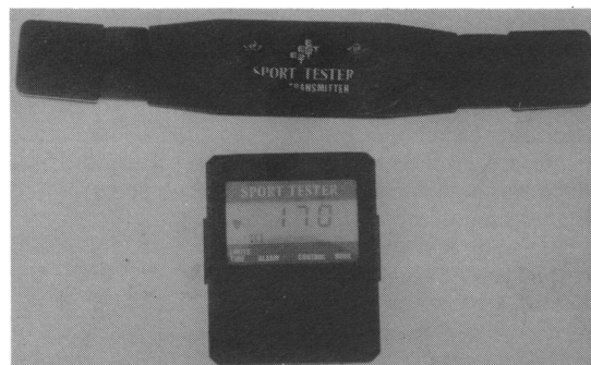
Fig. 1 The 'Sport-tester', showing the transmitter (top) and the receiver (bottom).
