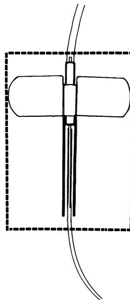
Figure Diagram illustrating needle feeding line assembly, with position of elastoplast indicated by dotted line.
