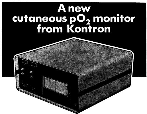
This new technique is being used on an increasing scale to supplement blood gas analysis of high risk neonates by continuously monitoring and recording cutaneous  $p0_2$  via a temperature-stable, non-invasive sensor.
