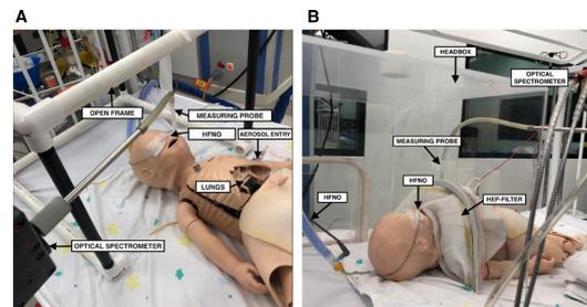
**Figure 1** Infant mannequin in (A) no headbox (open frame), (B) headbox with a HEP-filter attachment at the neck opening. The filter was removed in the open headbox setup, and a blanket was used at the opening for the headbox-blanket setup. HEP-filter, high-efficiency particulate filter; HFNO, high-flow nasal oxygen.
